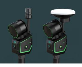
LiGrip O2 is the next-generation flagship handheld SLAM LiDAR scanner developed by GreenValley International. This all-in-one device integrates a laser scanner, panoramic cameras, visual SLAM cameras, and a GNSS antenna, enabling high-precision, all-directional data acquisition without limitations of time or environment.
