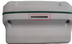
Measure the antenna height from two directions using a steel tape measure. If the error is less than 3mm, calculate the antenna height using the average value.
