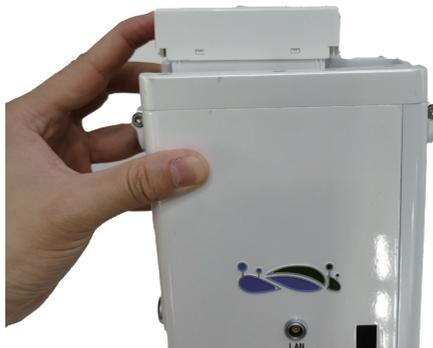
2. Installing battery box into the vehicle kit battery compartment, and securing the screw and battery latch
