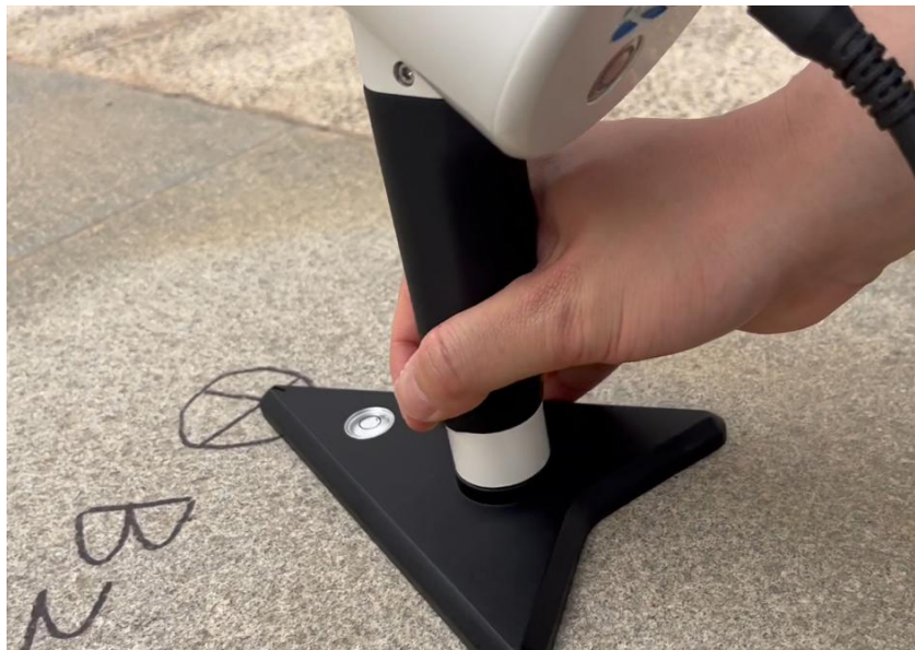
Figure 5-15 GCP collection (Align the "cross" hole with the control point)
