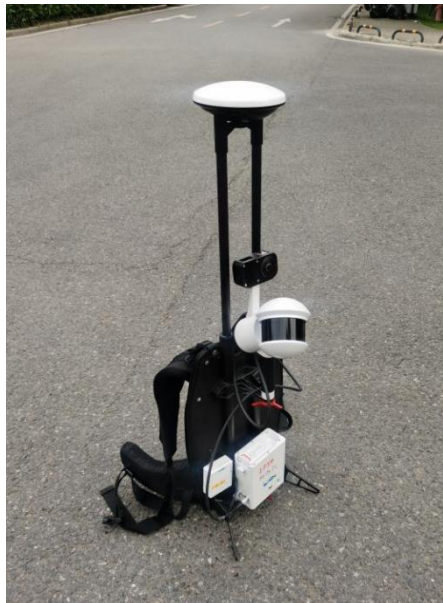
Figure 5-29 Slowly remove the device and place it on the ground when the collection stops
