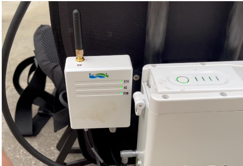
Figure 5-24 Indicator always on in case of successful RTK link configuration
