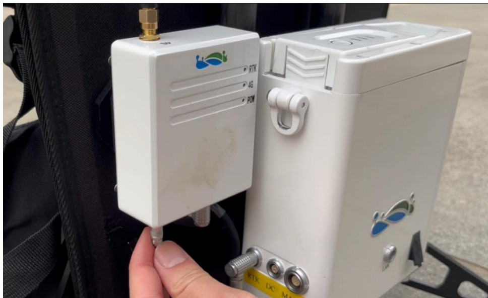
Figure 2-12 Inserting GNSS feeder cable into the GNSS interface of the GNSS module
