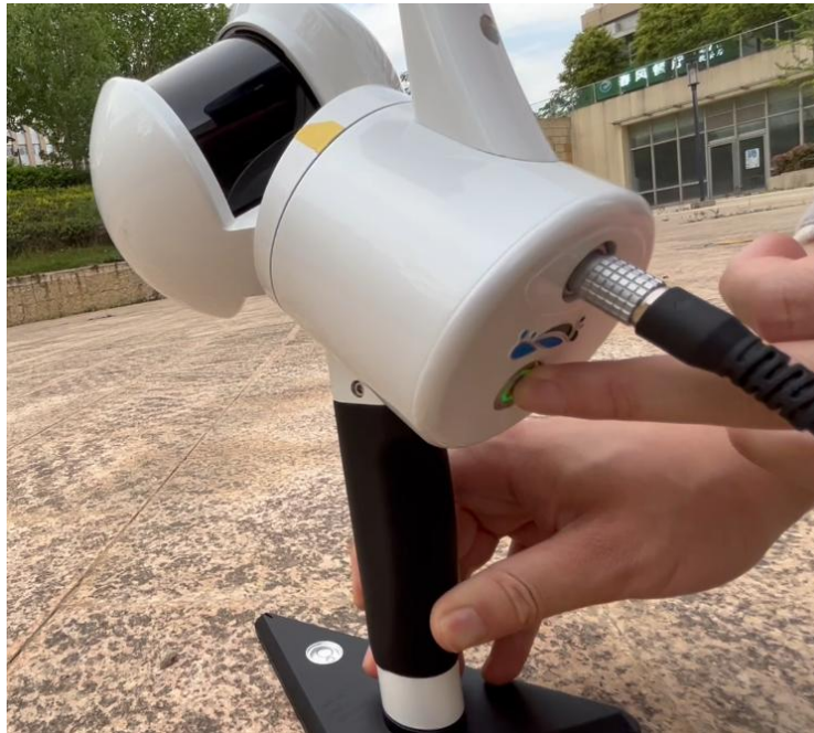
Figure 5-13 Long-press the button for initialization
