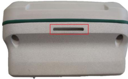
Figure 4-3 Instrument height measurement position
