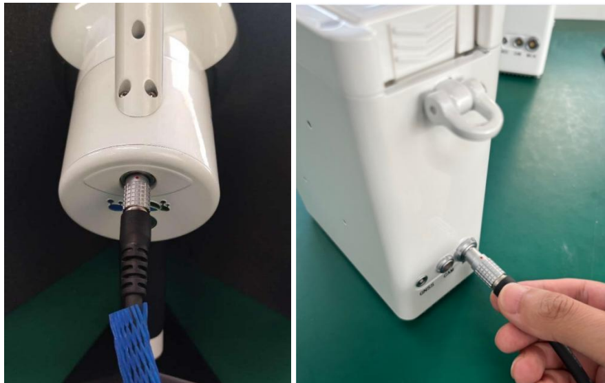
Figure 2-3 Connecting the handheld main unit to the battery compartment (MAIN port) by using the power cable
