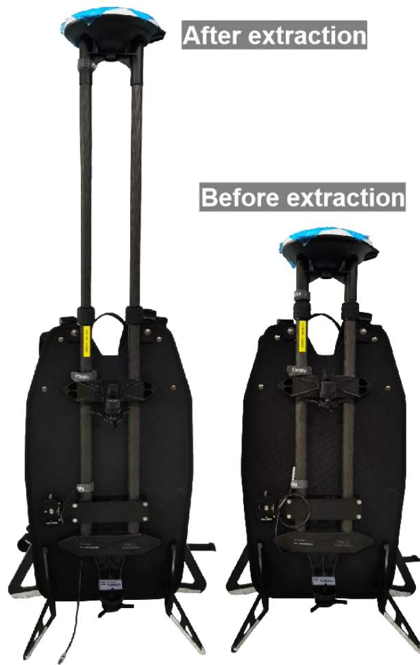
Figure 2-9 Comparison of backpack kit (before and after withdrawal)
