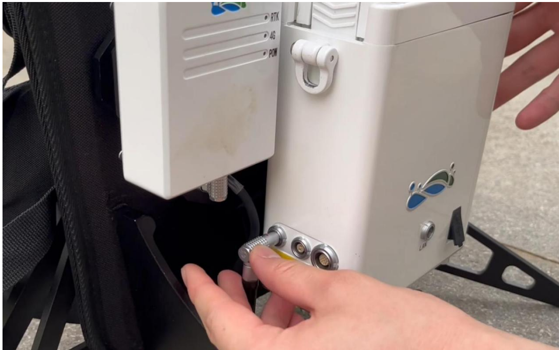
Figure 2-13 Inserting the RTK cable into the RTK interface of the main unit box and GNSS module respectively
