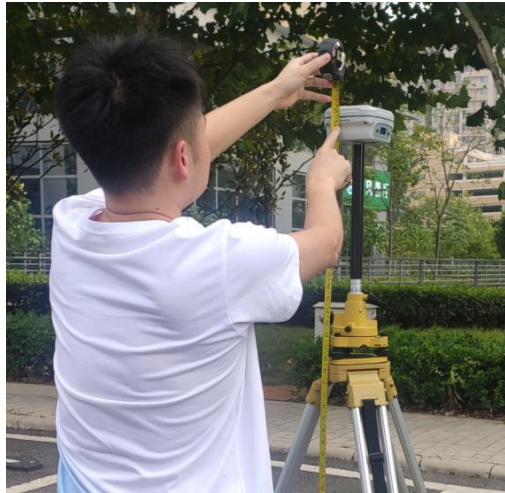
Figure 4-2 Instrument height measurement
