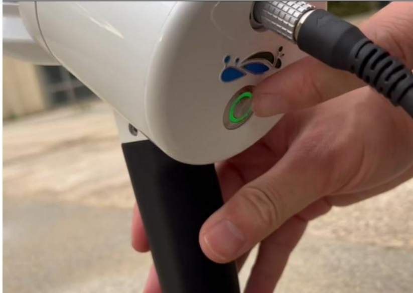
Figure 5-16 Short-pressing the green button (indicator: slow flash-> fast flash (collecting GCP); Fast Flash-> Slow Flash (finished))
