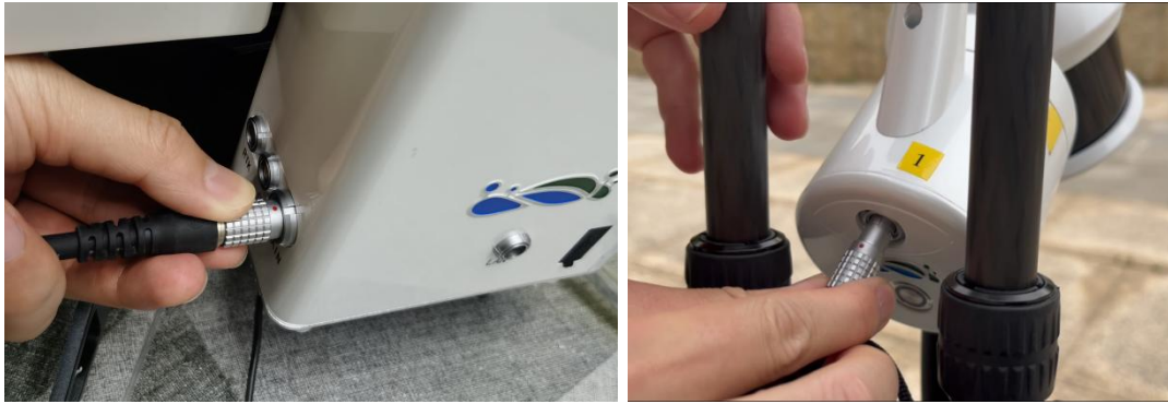
Figure 2-15 Connecting the power cable (MAIN port)
