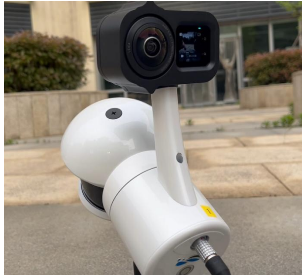
Figure 5-17 Camera automatically stopping recording when the laser rotation ends
