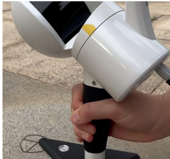
Figure 5-7 GCP collection (Align the "cross" hole with the control point)
