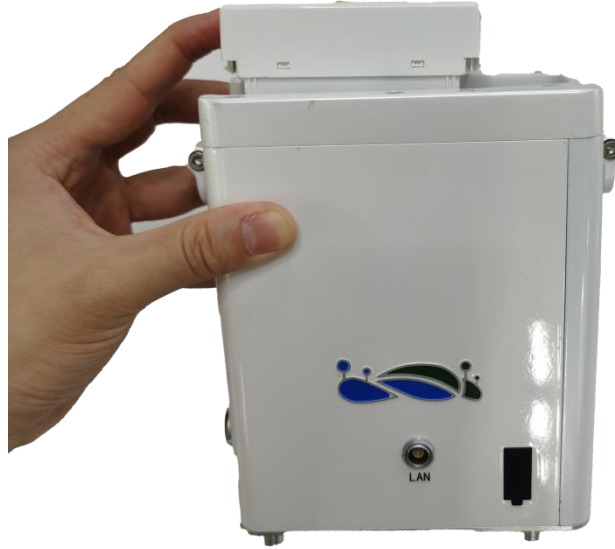
Figure 2-2 Inserting the B58 battery
