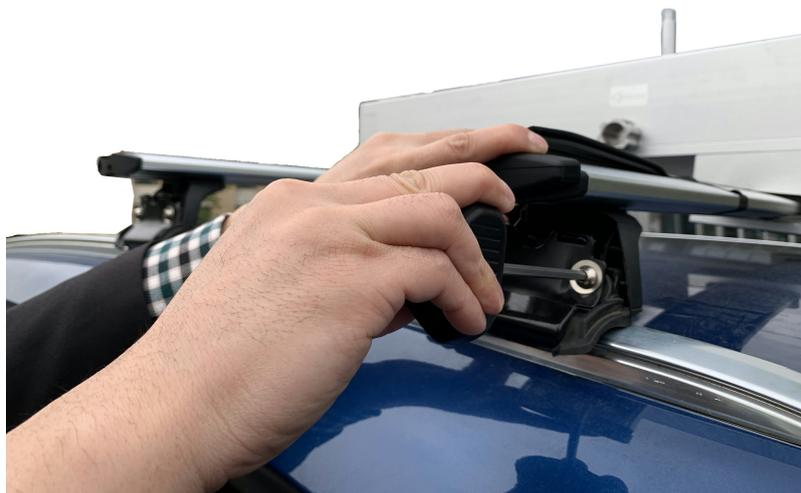
Use hexagonal screwdriver to lock the luggage rack in position.
