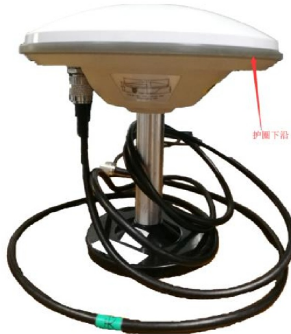
Base Station Antenna
