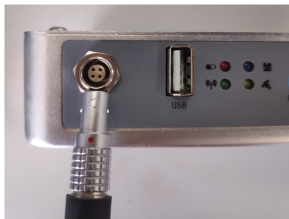
Base Station Power Cable
