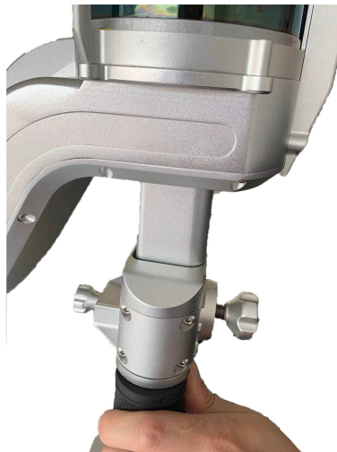
Mount the scanner on main body
