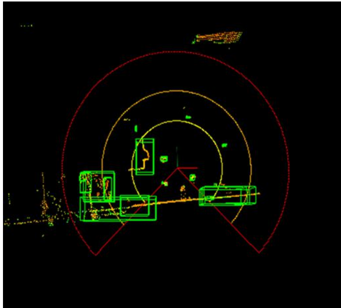
Figure 5 Obstacle point cloud in annular areas
