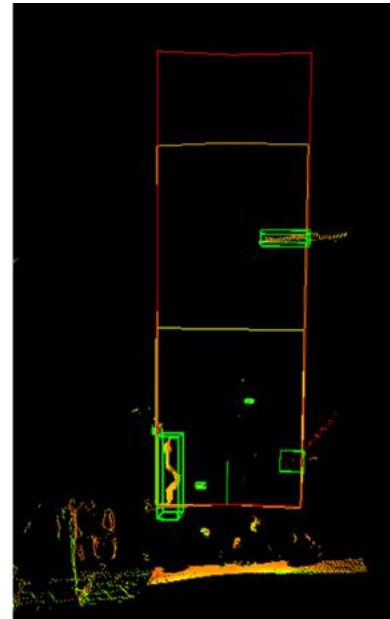
Figure 6 Obstacle point cloud in polygonal areas
